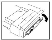
3 When the indicator on the [Start] key lights up in green, insert one page of the document face down into the single-sheet feed tray.
